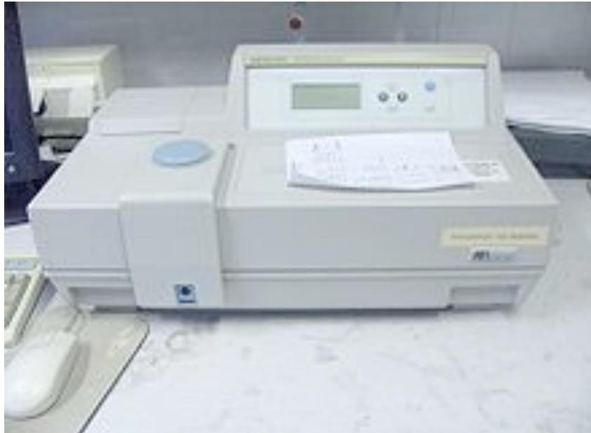
Spectrophotometer is a photometer that can measure the intensity as a function of the light source wavelength. The device measures absorbance using the following mathematical relationship:
